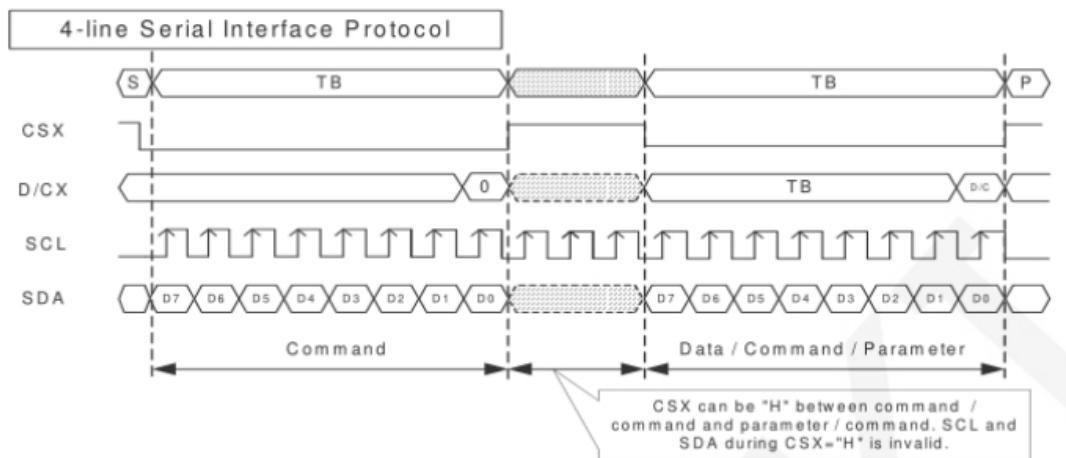
CSX is a slave chip select, and the chip is enabled only when CSX is low. D/CX is the data/command control pin of the chip. When DCX is low, the command is written. When it is high, the data is written. SCL is the SPI bus clock, and each rising edge transmits 1 bit of data; SDA is the data transmitted by SPI, and it transmits 8-bit data at a time. The data format is as shown below:
